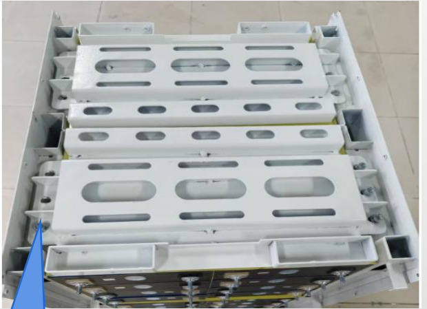
After tightening the electrical connection screws, check with a torque wrench and mark them.
